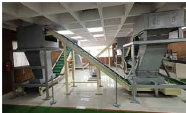
Transfer Chute Setup to handle Alternate Fuels Installed at NCB Ballabgarh
