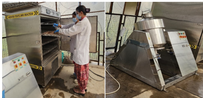
Aerated Static Bed Reactor (Left); and Pre Mixer (Right)
